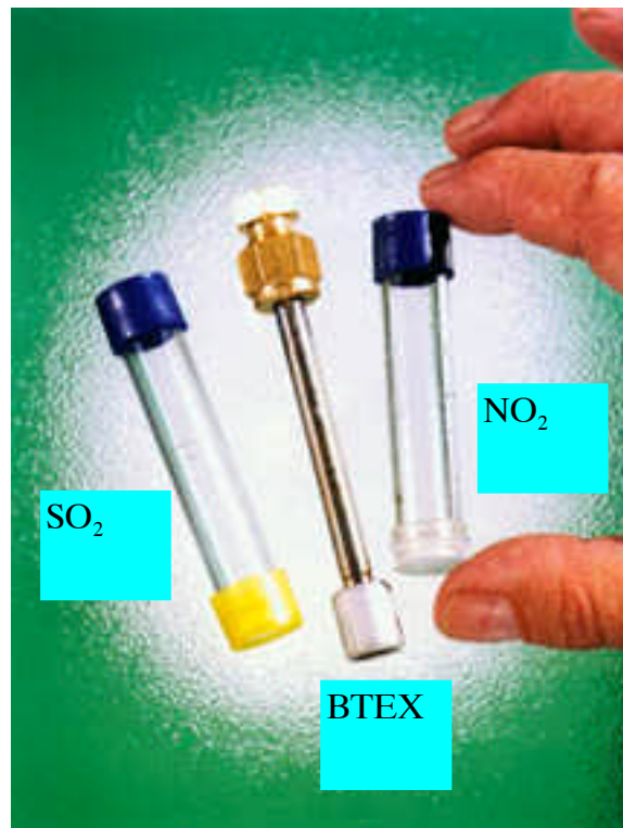
Photograph 5: Examples of SO 2 , VOC (eg Benzene), and NO 2 diffusion tubes.
